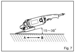
During the break-in period with a new wheel, do not work the grinder in the A direction or it
