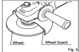
By slightly loosening the setting screw, the wheel guard can be turned and set at any desired angle for maximum operational effectiveness. Ensure that the setting screw is thoroughly tightened after adjusting the wheel guard.
